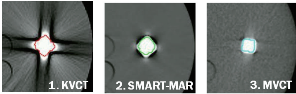
Fig. 2. Axial CT image with Metal B(1×1×1 cm) in Head & Neck In House Phantom. 1 : Auto contouring Metal B on KVCT, 2 : Auto contouring Metal B on MAR CT 3. Auto contouring Metal B on MVCT
