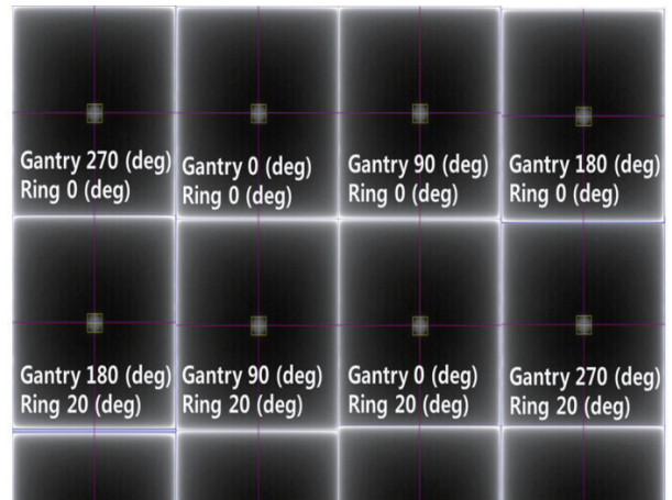
Fig. 6. A series of beam-eye view(BEV) images were obtained at the 12 gantry and ring angles using the MV imaging panel.
