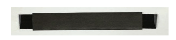
Fig. 11. CNT-coated fabric sensor
