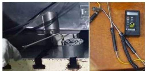
Fig. 2 Product attachment temperature measurement
