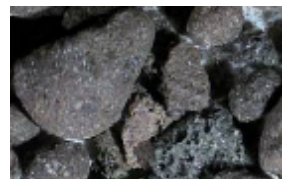
Expanded clay (magnified 9.45x)
