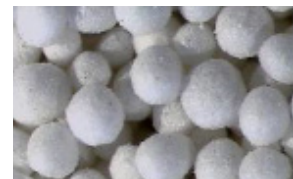
Expanded glass granulate (magnified 30x)
