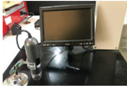
Fig. 3. USB microscope in the experiment.
