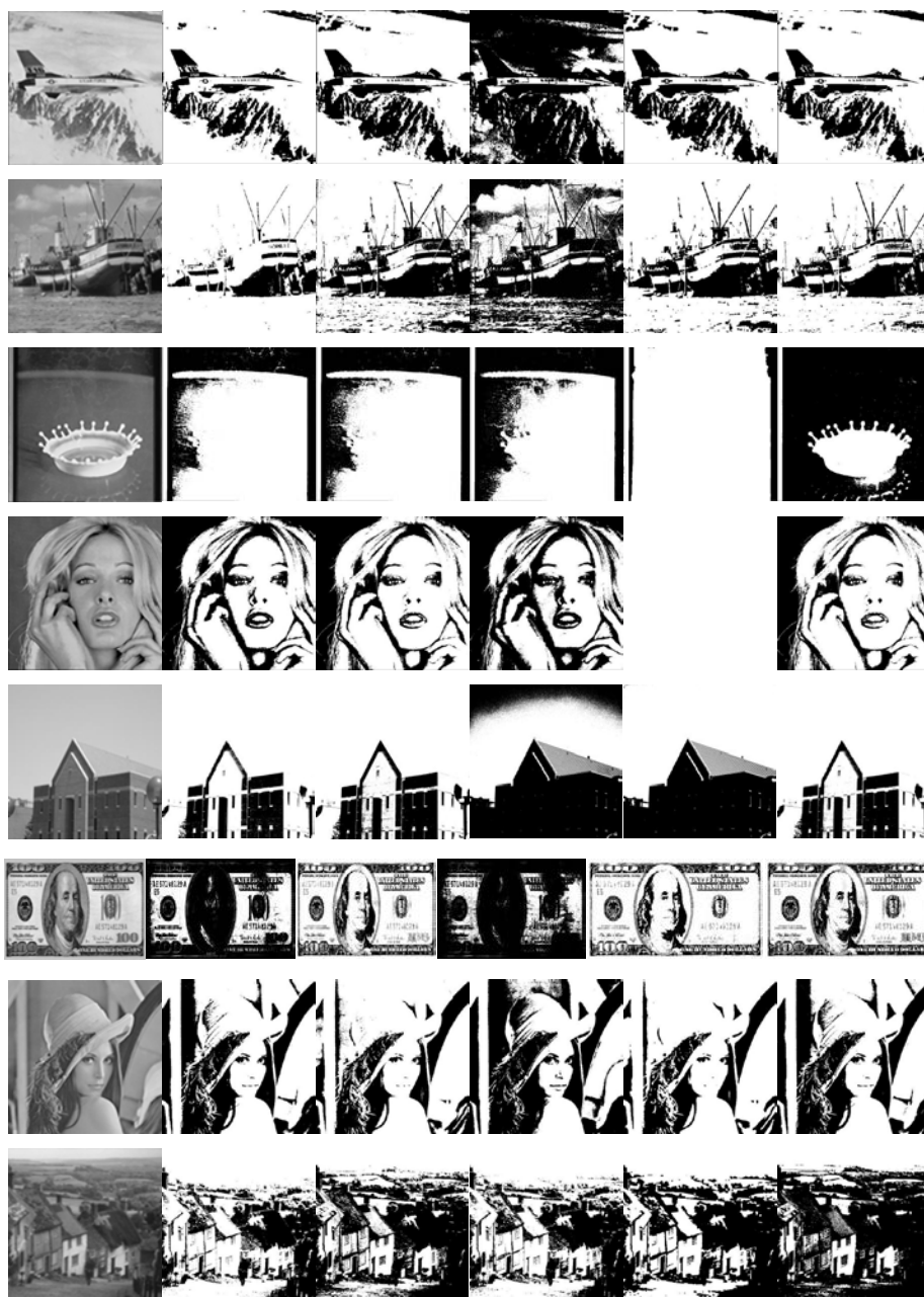
Fig. 5. Thresholding results of test images using different methods. From left to right: original images, the results obtained by 2D KSW, GLSC KSW, 2D-D KSW, GLGM KSW and our approach.
