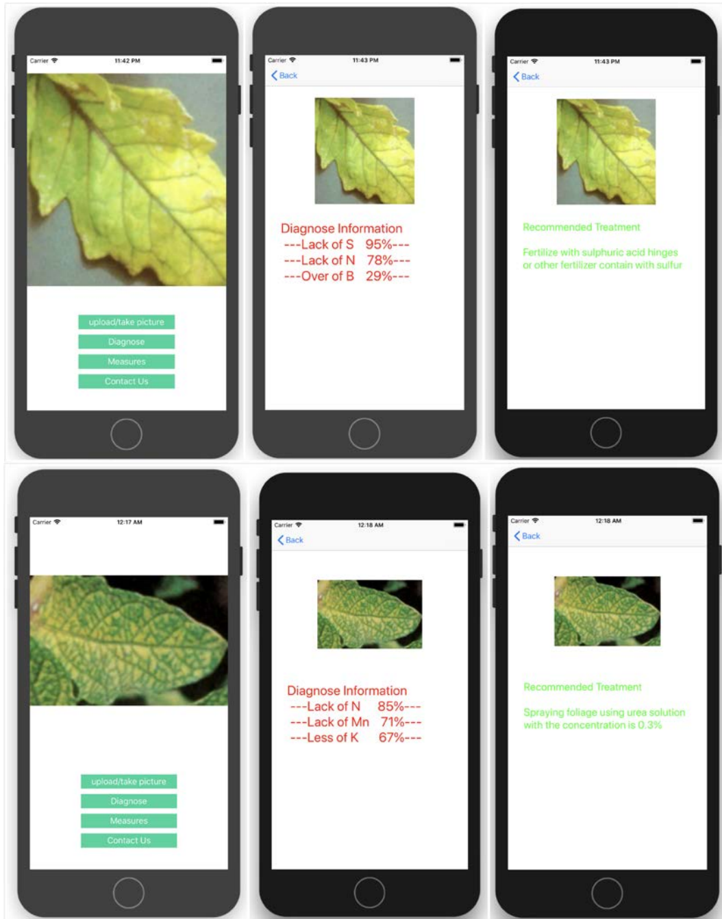
Fig. 10. Partial results of the application on mobile. User take a photograph by camera (left); the application returns top three results (middle); at the same time the application give some advice to user (right).
