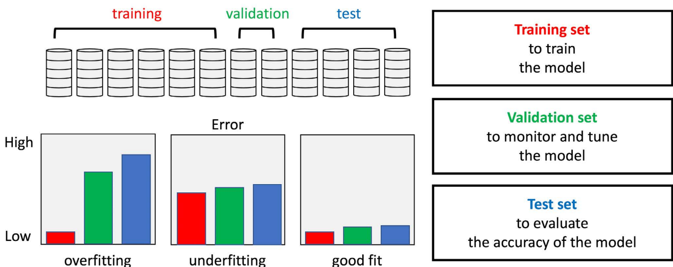
Fig. 3. Splitting data into training, valid, and test sets is generally recommended so as to avoid overfitting and evaluate the performance objectively. The optimally fitted network shows similarly good performances for all three data sets.
