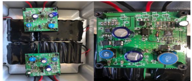
Fig. 13. Actual circuit picture of VVSM.
