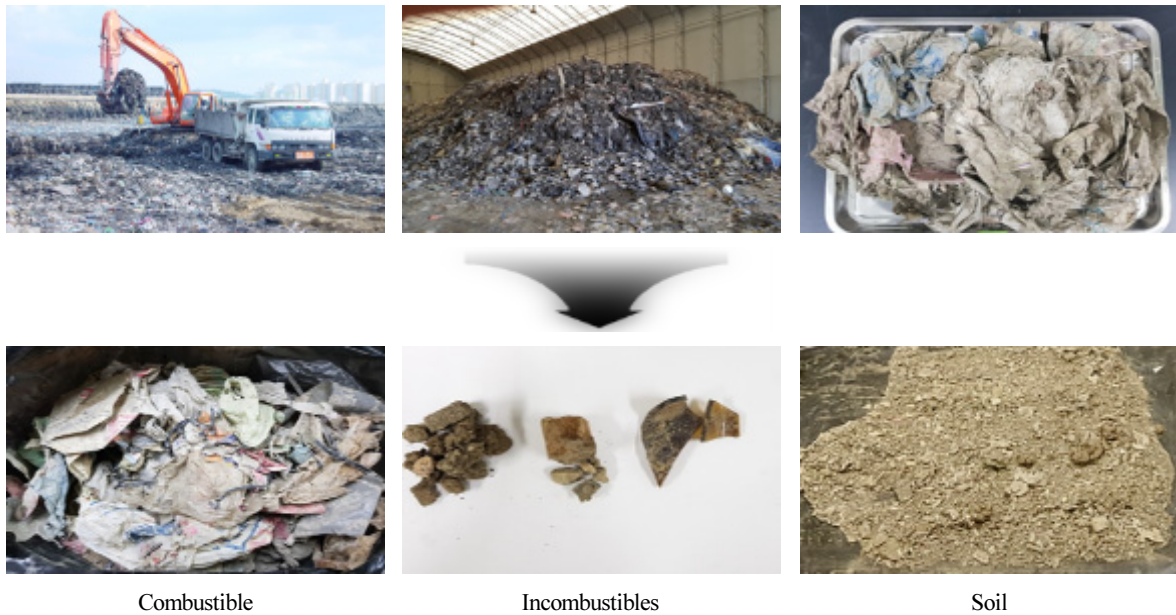
Fig. 1. Separation of excavated screened combustibles.
