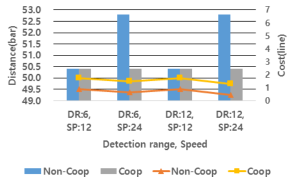
Fig. 6. Sailing distance and cost when safety domain is 0.5 nm.
