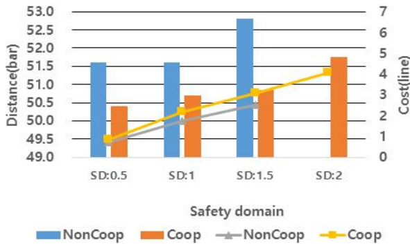
Fig. 10. Sailing distance and cost depending on the size of the safety domain.
