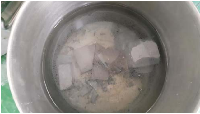
Fig. 11. Sea water curing in 14day(OPC)
