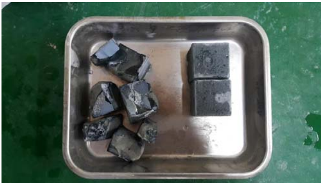
Fig. 12. Sea water curing in 14day(NGB)
