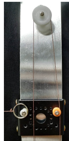
[Fig. 9] Left rail, a cart, an anchorage and a pulley
