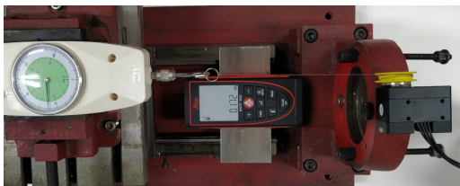
[Fig. 14] Experimental setup for measurement of cable tension, and displacement
