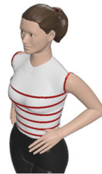
[Fig. 3] Concept of the cable driven size and stiffness realization for armhole, chest and waist
