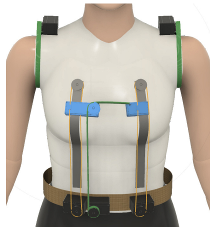
[Fig. 4] Haptic upper garment design
