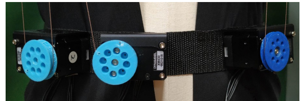
[Fig. 8] A Belt with cart u/down drive motor and a cable drive motor
