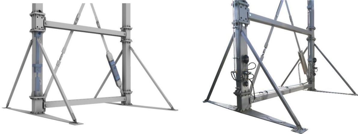
Figure 7. Adaptive frame, a full-scale prototype; Left: Visualization with adaptive elements (blue) Source: IKTD/ILEK; Right: Photography of frame at ILEK platform Source: ILEK.
