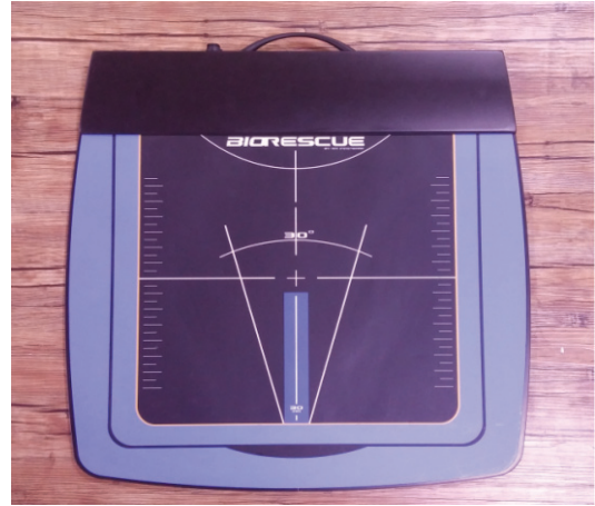
Fig. 1. Balance measure system (Biorescue, RM Ingenierie, France).
