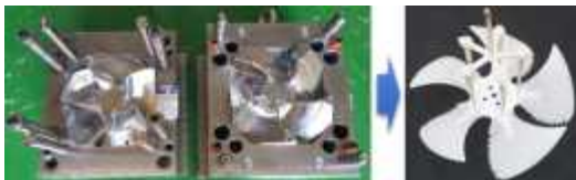
Fig. 10 Final mold and injection molded axial fan
