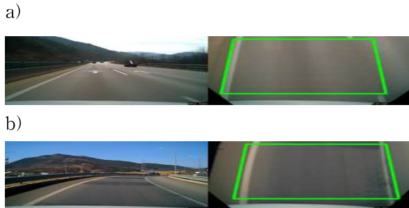
Fig. 7 Annotation of driving data with top-view transformation a) on a straight lane and b) on a curved lane
