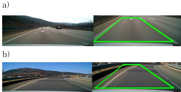
Fig. 6 Annotation of driving data without top-view transformation a) on a straight lane and b) on a curved lane
