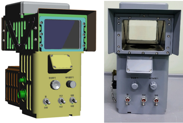
FIG. 12. Appearances of the developed optical sighting system.
