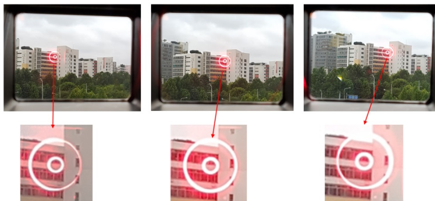
FIG. 14. Photographs depicting how an external object and virtual image of the reticle can be seen in a superimposed state anywhere on the observation window in the developed optical sighting system.
