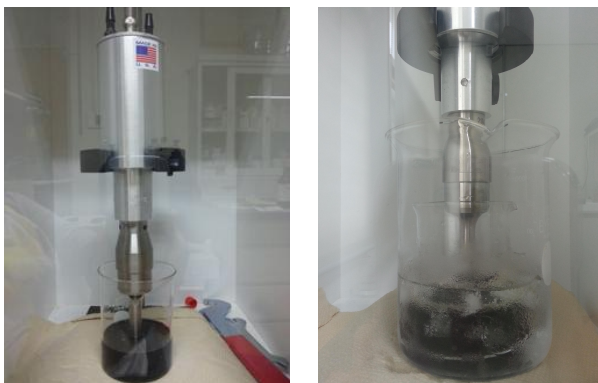
Figure 1. Photographic images of tip sonicating process used for the dispersion of SWCNT in the deionized water
