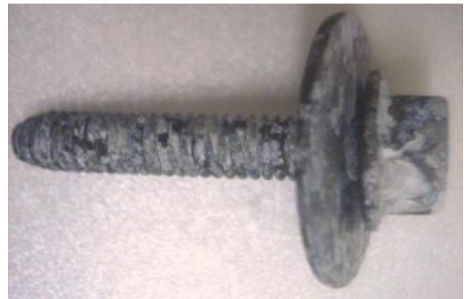
Fig. 1 An example of white storage stained steel bolt
