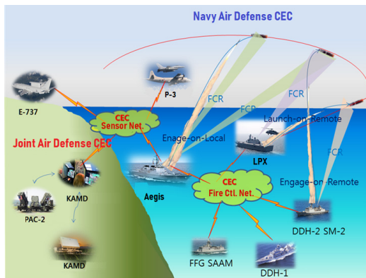
<Figure 4> ROK CEC Operation Structure
