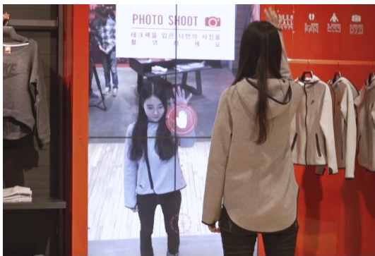
<Figure 2> User Stands in Front of the Interactive Mirror and Makes a Hand Gesture to Proceed to the Next Stage
