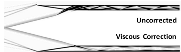
Fig. 12. Numerical Schlieren Images of Conical Intake with/without Viscous Correction
