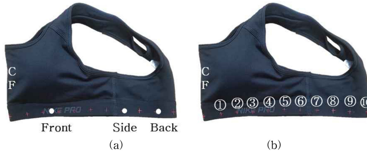
Fig. 2. Measurement positions of experimental sports brassiere: (a) Measurement location of pressure; (b) 3D length measurement.
