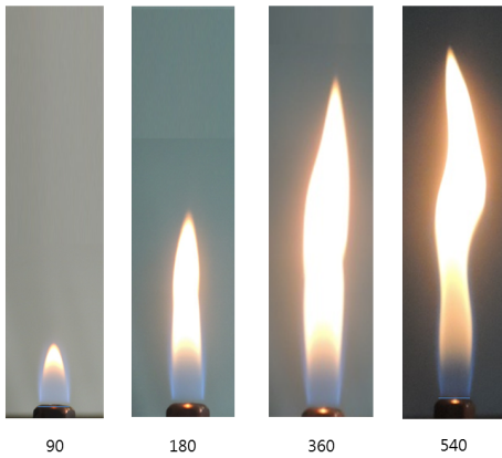
Figure 3. Direct photos of methane jet diffusion flames as increasing fuel flow rate. The numbers below each picture indicates the flow rates (sccm) of methane.
