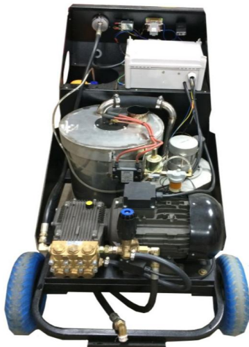
Fig. 1 High temperature/high pressure washer in which the low pressure boiler supplies hot water
