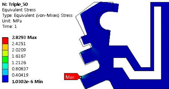
(b) Main lip's oil side angle \alpha = 50^\circ
