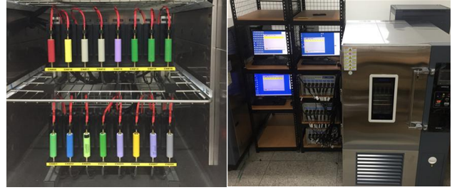
Fig. 7. Single cell experiment equipment.
