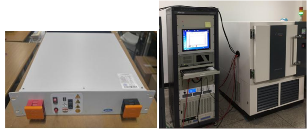
Fig. 8. Battery pack experiment equipment.
