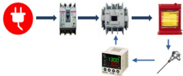
[Figure 4] A heating unit in which the temperature control unit is separated by sensors and controls and switches.
