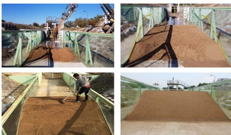
Fig. 4. Construction of levee model.
