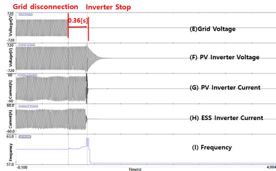
Fig. 4 The results for islanding detect of case 4 (R load capacity: 0 [kW])
