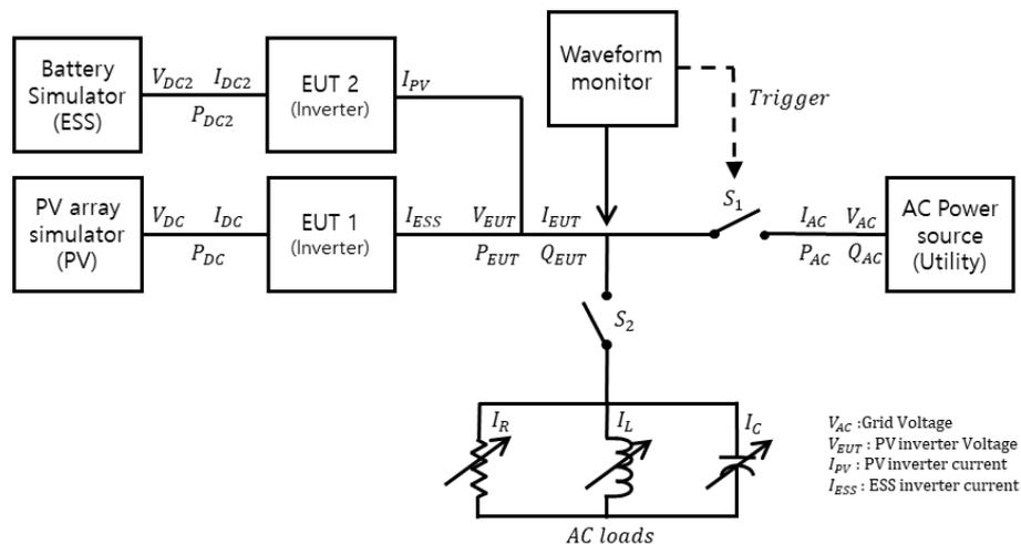
Fig. 1 Configuration diagram for islanding detect test
