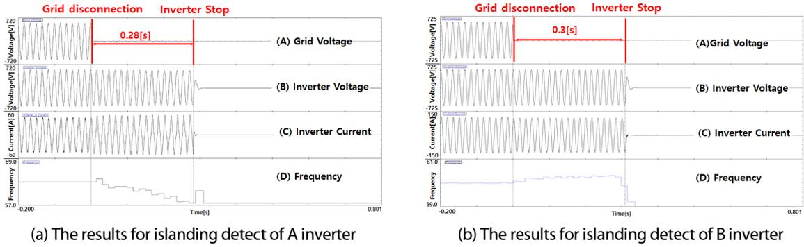
Fig. 2 The test results for islanding detect of one inverter
