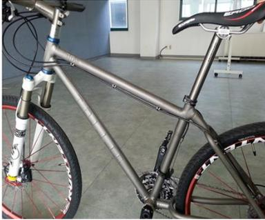
**Fig. 11 Appearance of a titanium bicycle using a Ti-3Al-2.5V joint structure fabricated by the SHF/DB process.**
