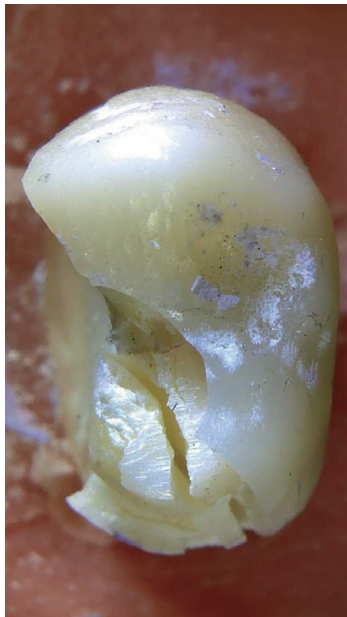
Fig. 2. Irreparable fracture of the monolithic zirconia crown and the tooth under a digital stereomicroscope (40×) for the shoulder margin design (Code V).
