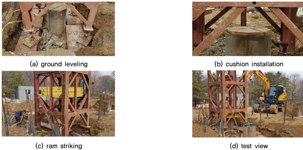
Fig. 2. Dynamic loading test procedure
