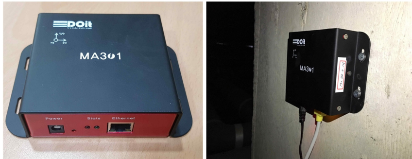
Fig. 4. Seismic wave measuring device to communicate with ICU
