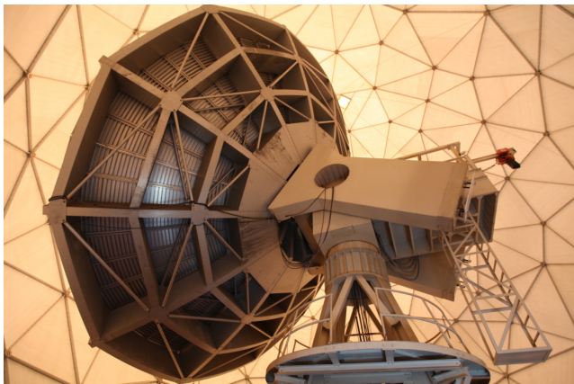
Figure 1. The TRAO 13.7-meter radio telescope.
