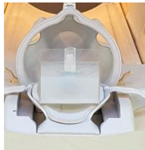
Fig. 2. 3T Phantom is acquired from the head coil of 3.0T MRI Equipment.
