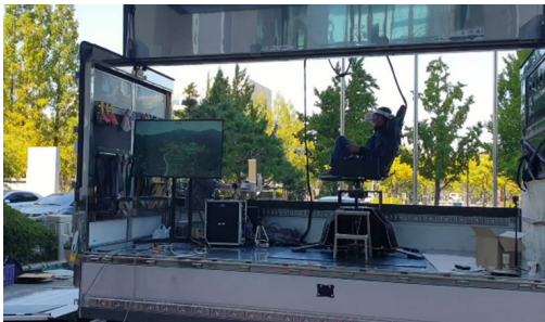
(b) The drone operator on the simulator moved by the IMU data from the remote site drone in location B
