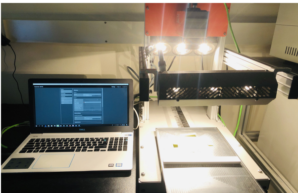
Fig. 3. Hyperspectral camera in laboratory
