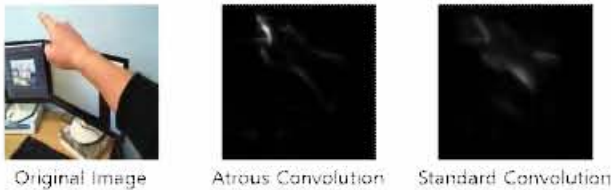
Figure 7. Original image, feature map with Atrous convolution and feature map with standard convolution
