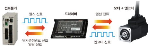
Fig. 12. Conceptual Diagram of Autronics AiS Step Motor Control System.
