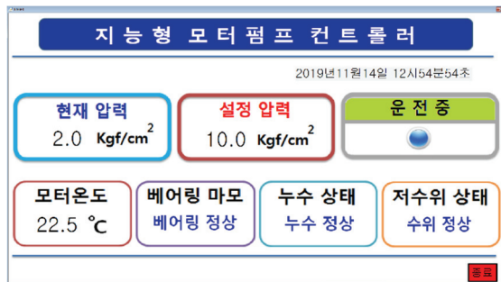
Fig. 7. SCADA Monitoring System.
