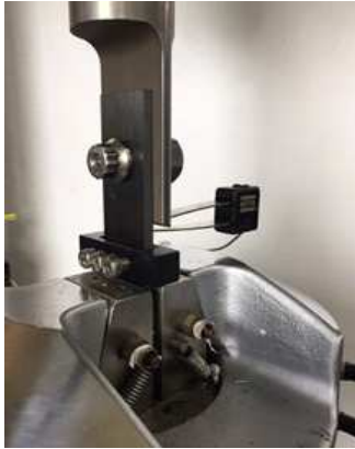
Fig. 6 Bolted Composite Joints Tensile Test
