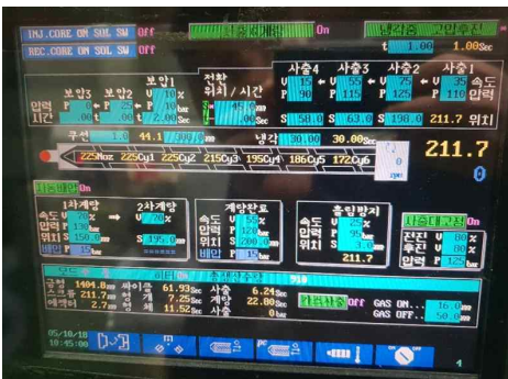
Fig. 10 Injection machine try out conditions
