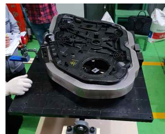
Fig. 13 SPL Warpage measurement
