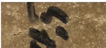
Fig. 5 Fine surface cracks on the specimen
