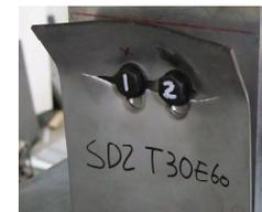
(c) Additional tensile fracture toward plate edge in Step ③
