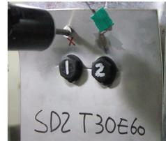
(b) Tensile fracture between two bolts in Step ②
