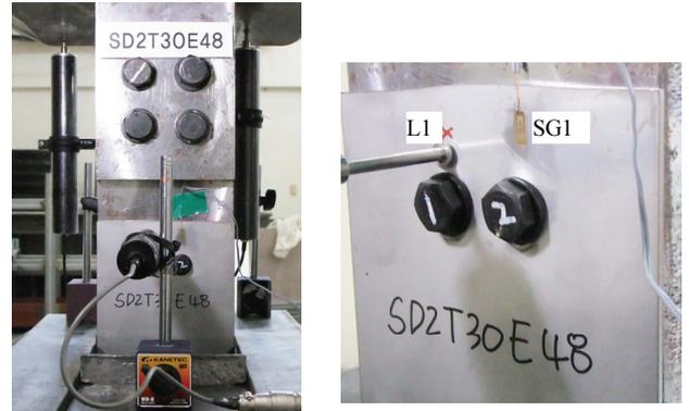
(a) Transducers(LVDTs) (b) Strain gauge for SD2T30 series
