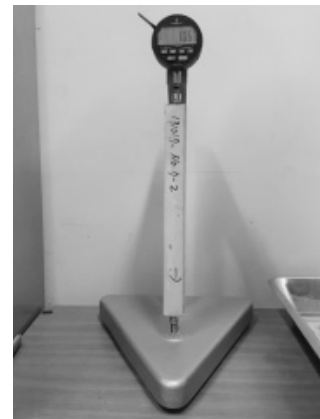
Fig. 4 Test setup of drying shrinkage.
