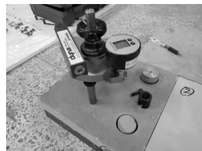
Fig. 5 Test setup of bonding
