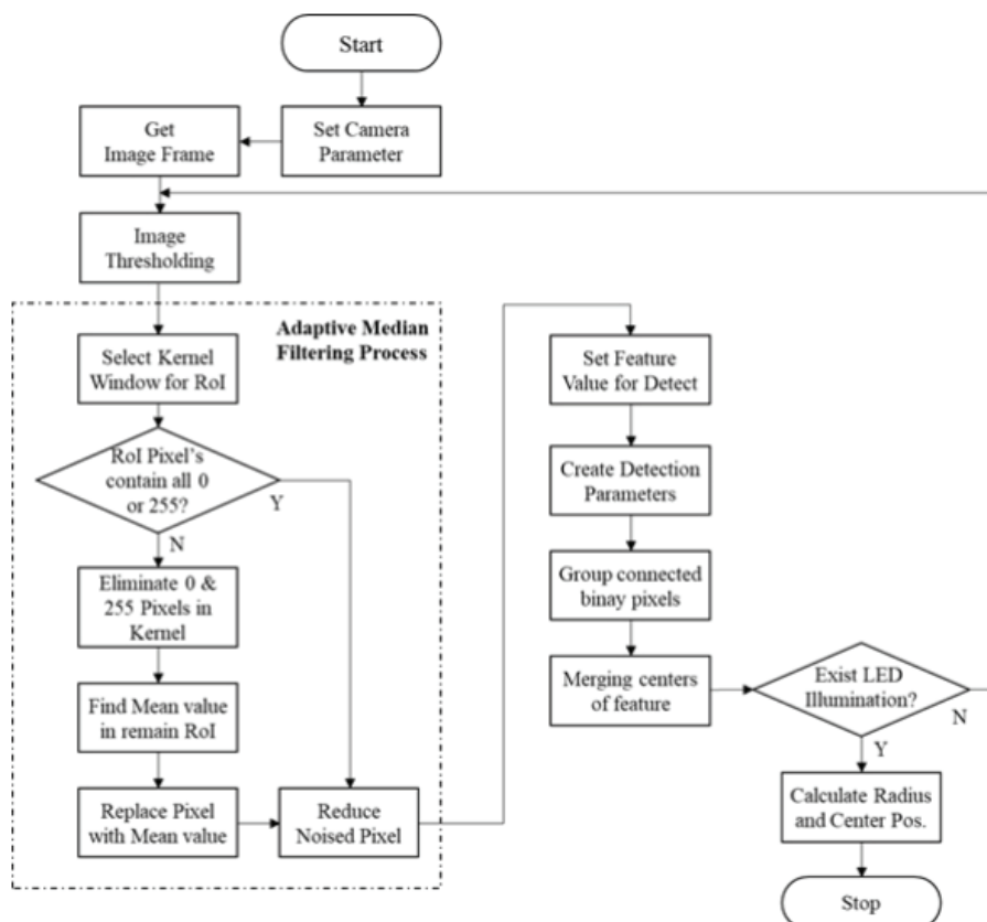
<Fig. 1> Adaptive median filter applied LED illumination detection algorithm
