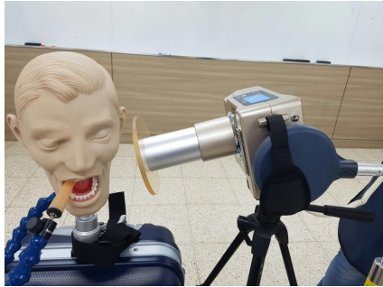
Fig. 3 A photograph of measuring the scatter ray
