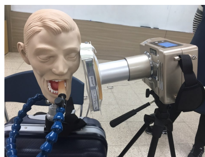
Fig. 2 A photograph of measuring the Dose area product
